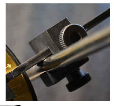
Lock plate secure on the support shaft
