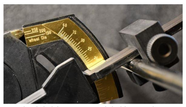
Dps Angle scale divided into 0,5 Degree and wheel diameter scale
