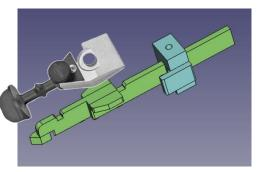
B. Set the wheel size on the Tool by loosening the centerplates locking screw, place the tool on the wheel and carefully move the centerplate down so the two 10mm metal shafts hit the wheel together with the centre point on the main-part. Three points should now rest against the wheel. Lock the centerplate with the screw on the backside.
