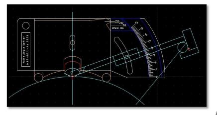
It is designed and drawn in Cad and the function is based on using two points (shafts) to self-center on a wheel and place the edge point of a ruler where the tip of the knife meets the grinding wheel. "The Edge of the Knife" The ruler in the Tool lies against the grinding wheel at the grinding point and rests against the USB support and shows the current angle on a degree scale.
