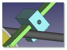
D. Gently press down the tool with the ruler so the shafts and ruler tip stay in place and touch the wheel surface. The ruler tip will always stay in the center regardless of what angle you set the ruler to or what size of wheel you have because of the vaulted house it is placed in.
