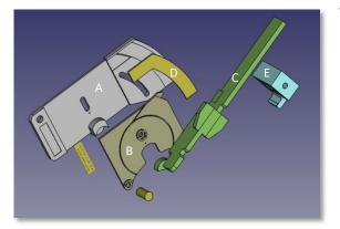
The parts of the tool are printed in a 3d printer and some parts are also milled in a CNC router to reach the fine tolerance required on some important dimensions. The scale is made in brass and engraved in a CNC milling machine when the tool is assembled and all parts are fixed in place. There are three moving parts that works together to achieve the function so dimensional accuracy is important.
