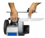
There is a simpel control function in the tool. Use an digital Angle cube to check the setting. Place an angle cube on top of the Tool and zero the cube. Then move the cube to the ruler and it will show
