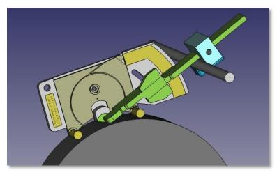
With this tool you can set the grinding angle of knives on a grinding machine with rotary grinding wheels or honing wheels from diameter 150mm and up to 250mm without using any calculator or caliper. There is no need to measure wheel size, usb height or projection length. It is self-adjusting in terms of wheel size and scale display. It also shows the current wheel size on a small scale. The ruler on the tool always hits the right point on the
