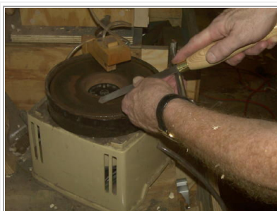
Figure 4: Sharpening the Spindlemaster with a modified Makita wet grinder featured in the February, March and April issues of More Woodturning and the authors web site.
