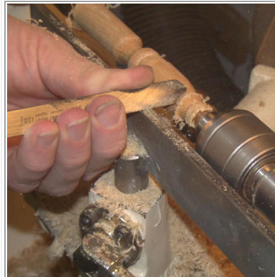
Figure 8: Planing a swell with the Spindlemaster. You may be able to see the burnishing left by the tool even with newspaper reproduction.
