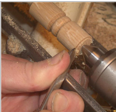
Figure 12: Plunge cutting end grain seen from above.
