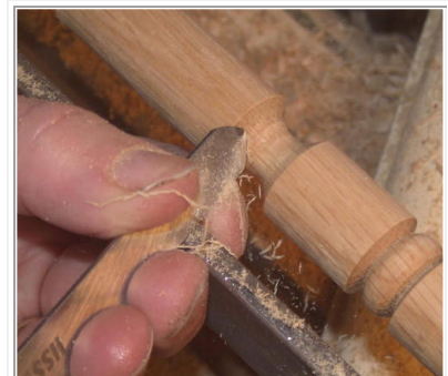
Figure 16: Cutting a cove seen from above.
