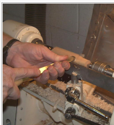
Figure 5: Taking a roughing cut on a 1 inch turning square with the Spindlemaster.
