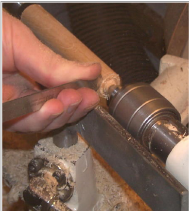
Figure 11: Plunge cutting end grain with the Spindlemaster.
