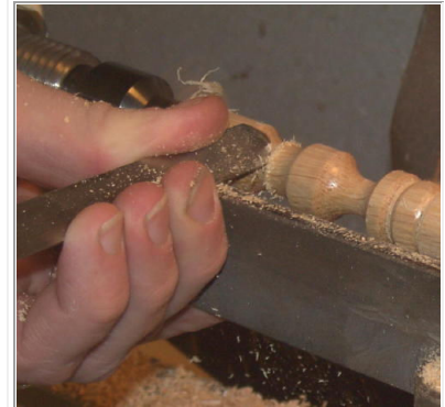
Figure 15: Cutting a cove with the Spindlemaster.
