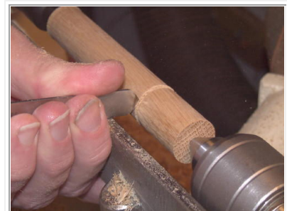
Figure 10: Plunge cutting a V with the Spindlemaster.
