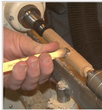
Figure 13: Rolling a bead with the Spindlemaster.
