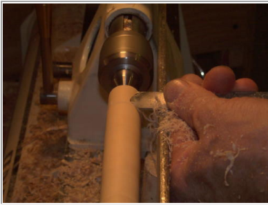
Figure 7: Taking a fine planing cut with the Spindlemaster. Note the fine shavings piling up on the authors hand.
