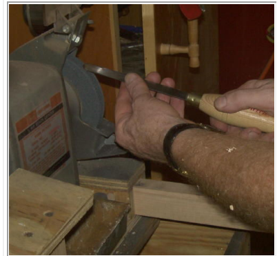
Figure 2: Sharpening the Spindlemaster with a bench grinder and sliding V-block.
