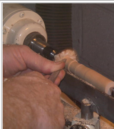
Figure 6: Taking a riving roughing cut with the Spindlemaster.
