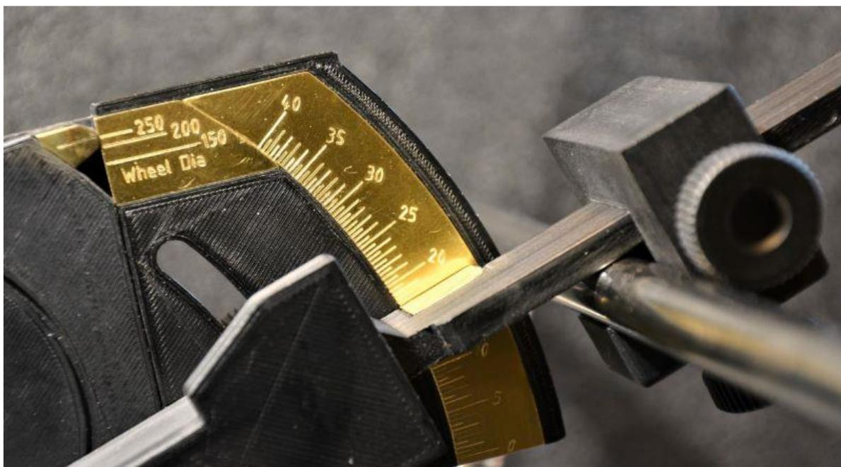
Dps Angle scale divided into 0,5 Degree and wheel diameter scale
