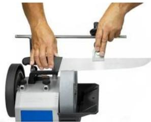
There is a simple control function in the tool. Use a digital Angle cube to check the setting. Place an angle cube on top of the Tool and zero the cube. Then move the cube to the ruler and it will show the angle value you have set.
