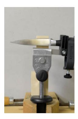
Photo five shows the slicing knife in the jig, also set to 139mm. Again, note the 139mm Protrusion pencil line above the knife.
