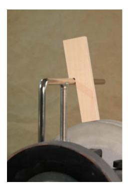
Photo eight shows the slicer knife in the jig ready for grinding. Setting the jig plus knife length to a Protrusion of 139mm and the top of the universal support to grinding wheel Distance to 80mm will produce consistend bevel angles with no further measuring.
