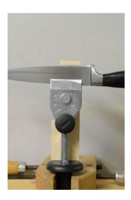
The sixth photo shows the chef's knife in the jig and set for 139mm Protrusion.
