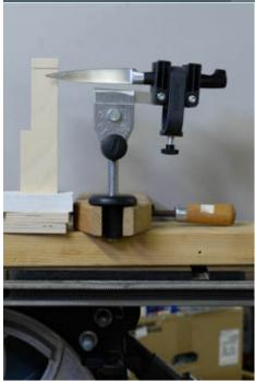
Photo one shows two jigs, one for the T7 and one for the T4. Note that the 139mm line is the same. The only difference between the two jigs is that the groove for setting the Distance between the universal support and the grinding wheel is 6mm longer (86mm instead of 80mm) This is because of the differences in diameter of the two wheels. Photo two shows one jig askew to illustrate the depth of the 12mm baltic birch plywood.
