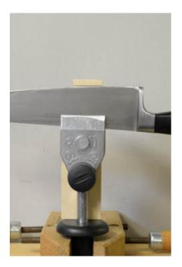
Photo seven shows the jig being used to correctly set the Distance between the universal support and the grinding wheel. No use of the anglemaster or black marker is required.
